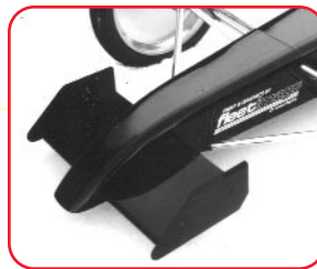
Wing tip profile "C" shown above on canard wings with outer tips.
