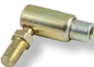
C90-044 Quick release ball joint 10-32 female X 1/4-28 male
